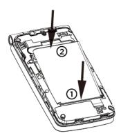
Align the contacts of the battery with the contacts in the phone.
